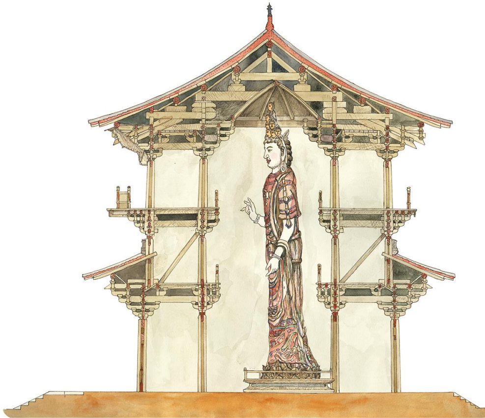
Figure 20. Cross Section of the Guanyin Pavilion at Dule Temple
